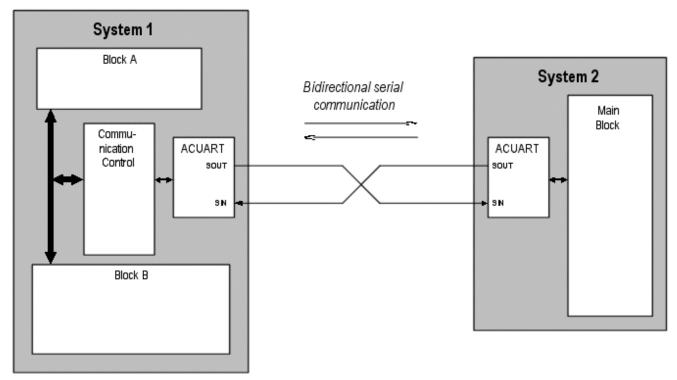
The ACUART can be used as an interface between systems with any architectures. The system uses the host interface of ACUART to control the communication.
