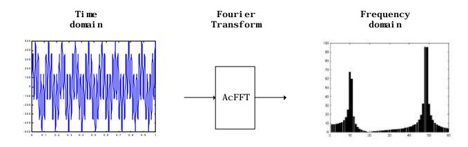
Fast Fourier Transform (FFT) is an algorithm to compute Discrete Fourier Transform (DFT) consuming O (N\*log<sub>2</sub>N) runtime (N - FFT size). DFT transforms time domain to frequency domain using equation:
