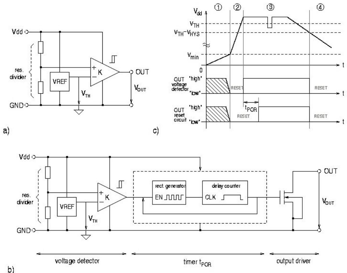
**Figure 8. General supervisory architectures: a) voltage detector, b) reset circuit, c) timing waveforms of a and b.**
