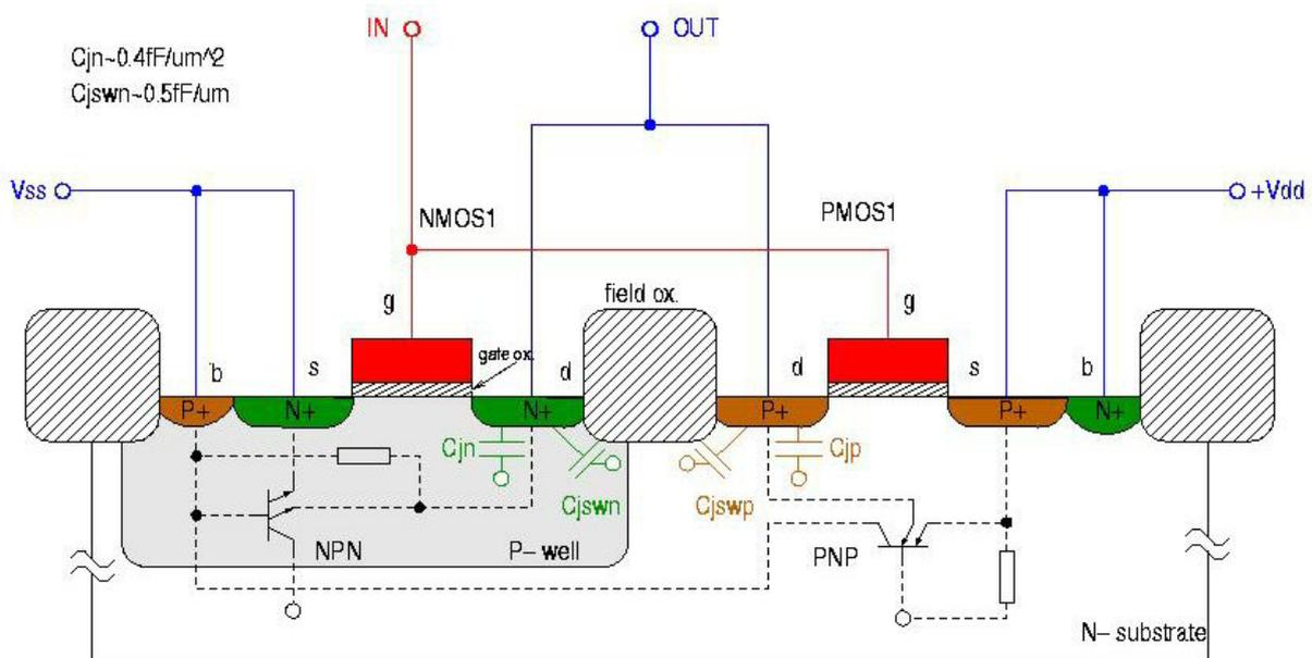
**Figure 1. Cross-section of a "bulk" CMOS inverter (including parasitic bipolar scheme for latchup).**
