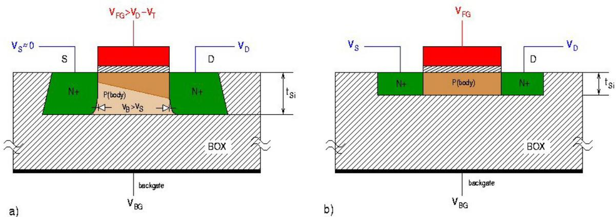
**Figure 5. a) Partially depleted (thick film) SOI MOSFET with kink effect; b) fully depleted (thin film) device.**
