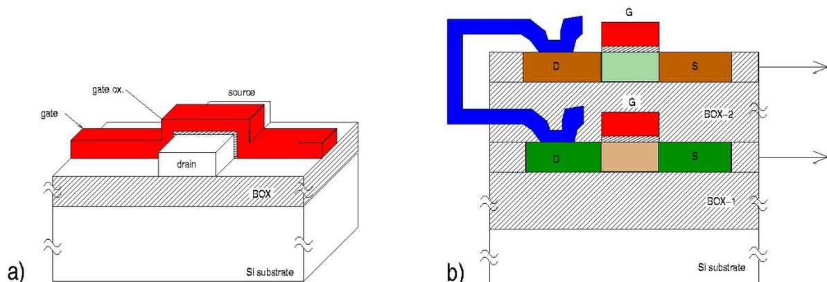
**Figure 4. Innovative 3D SOI devices: a) GAA MOSFET, b) stacked-transistor structure.**
