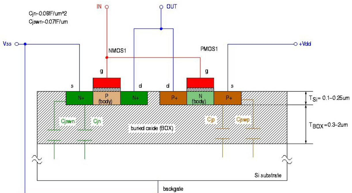
**Figure 3. Cross-section of a thin-film SOI CMOS inverter.**
