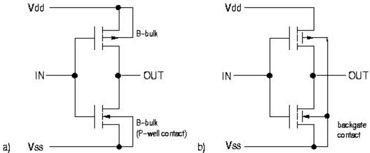
**Figure 2. Electrical scheme of bulk (a) and SOI (b) CMOS inverter.**
