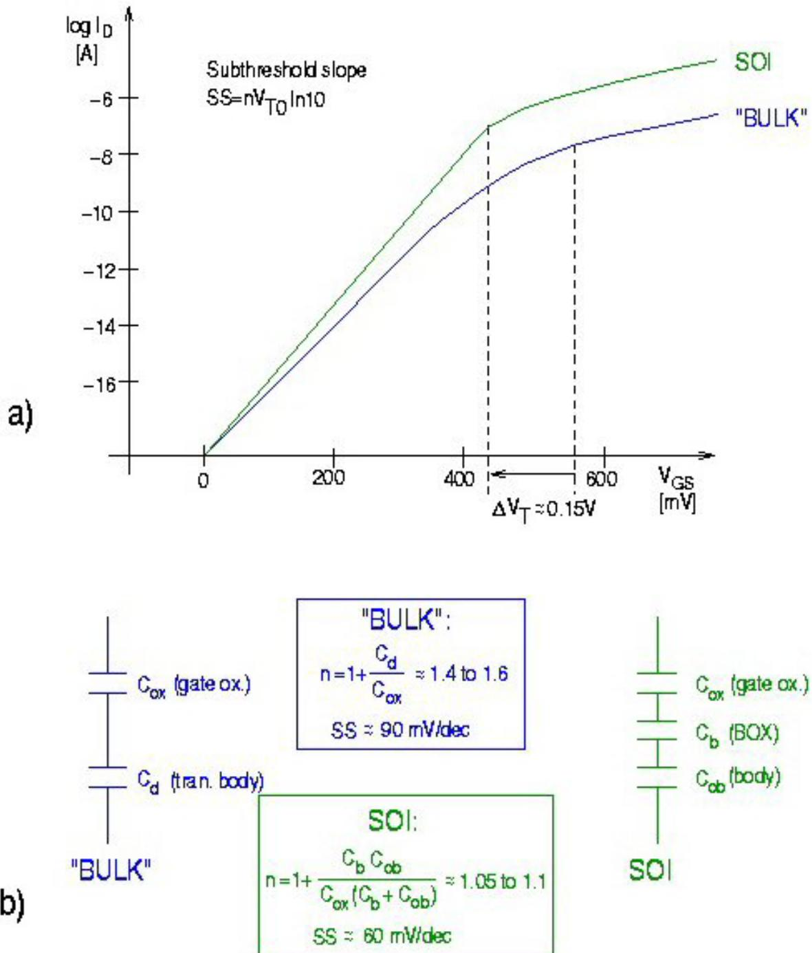
**Figure 7. Comparison of SS and VT for "bulk" and SOI: a) sub-threshold gate characteristics; b) corresponding equations.**
